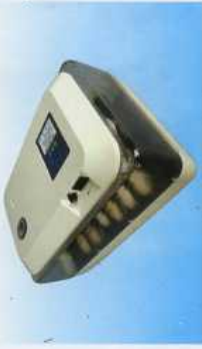
Fig. 4: pay attention that there's an egg turning rod in the transparent case at the upper part of device. The rod must insert into the channel of egg tray for the egg turning. The egg turning motor runs as long as the device is powered on. It runs one cycle every four hours so that it's very slow. The egg is turned once about every 4 hours.
